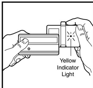
4. Press and hold the Remote Control X push button as you slowly slide the remotes across each other until the 372LM and 372LMC indicator light blinks very rapidly, indicating it has learned the code. (If Remote Control X is also a 372LM and 372LMC, you must press and hold its right push button.)
