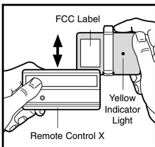
5. The right button is now sending the same identical coded signal as Remote Control X. This code will remain inside the 372LM and 372LMC until replaced with another new code by repeating steps 1-4 above, or by resetting to Security+®.
