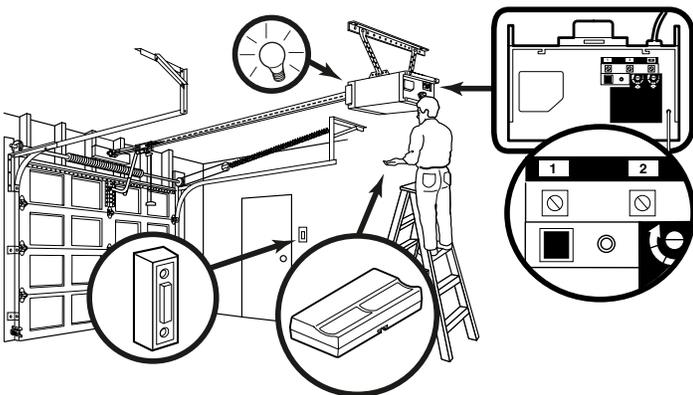
1. Press and release the “learn” button on the motor unit. The learn indicator light will glow steadily for 30 seconds.
