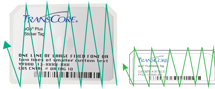
Figure 4 – Remove Air From Around Tag Chip
