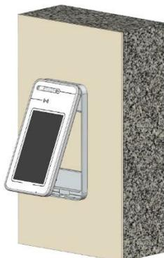
**Step 8** - Secure the VPS front panel to the case by reinserting the bottom screw.
